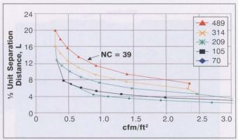
Figure 1 (left): Face-mounted deflector, 8 in. inlet, four way. Figure 2 (right): Spacing for 80% ADPI, 8 in. neck.
