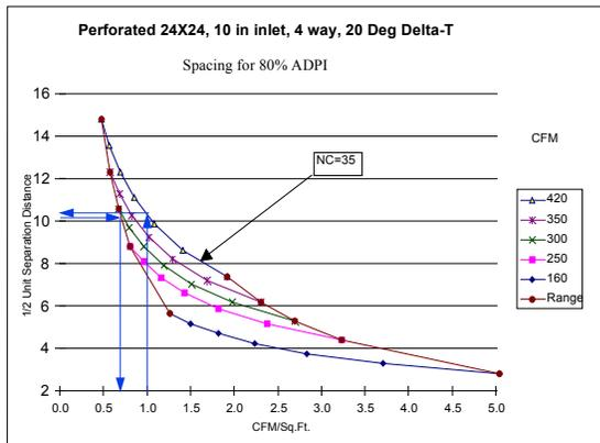
Figure 5: Selection using the envelope chart.
