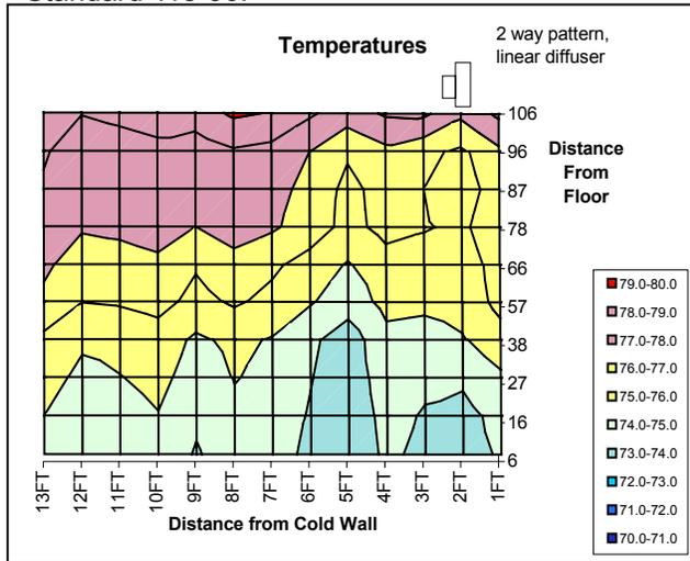
Figure 15: Perimeter Single Plane Temperature profiles.
