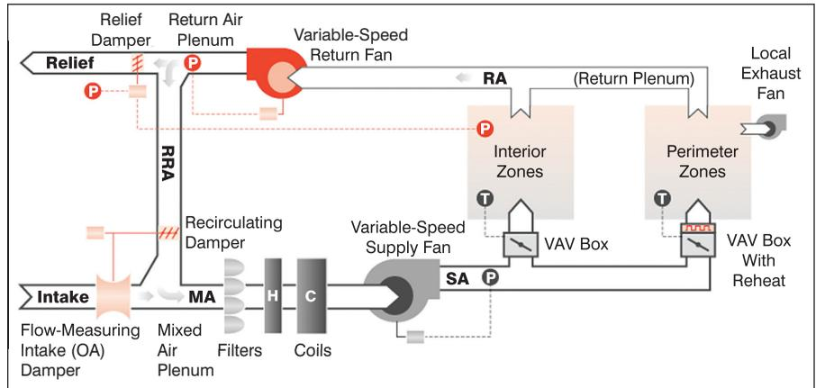
Figure 1: Variable air volume reheat system.
