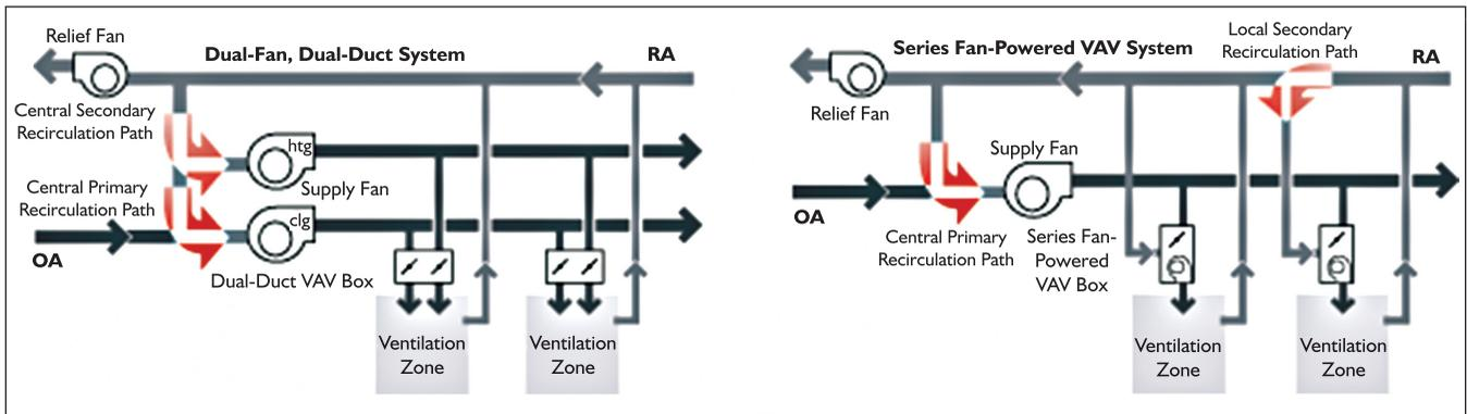
Figure 1: Dual-path, multiple-zone, recirculating ventilation systems.
