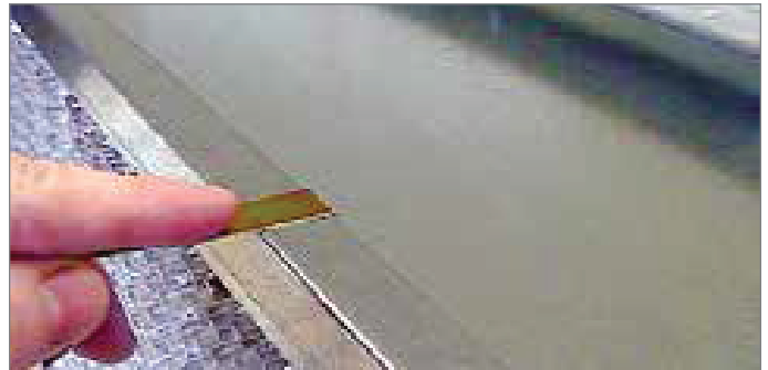
FIGURE 123 - POSITION PRE-FILTER IN FRONT OF FINAL FILTER
