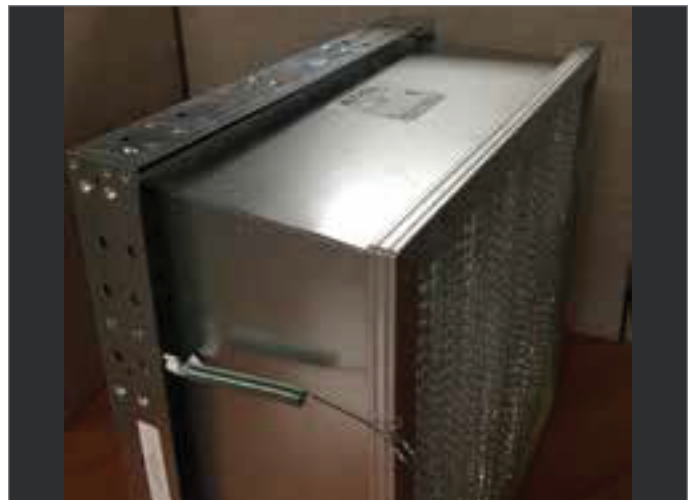
FIGURE 121 - SPRING LATCH PULLED AND FASTENED IN FILTER HOLE
