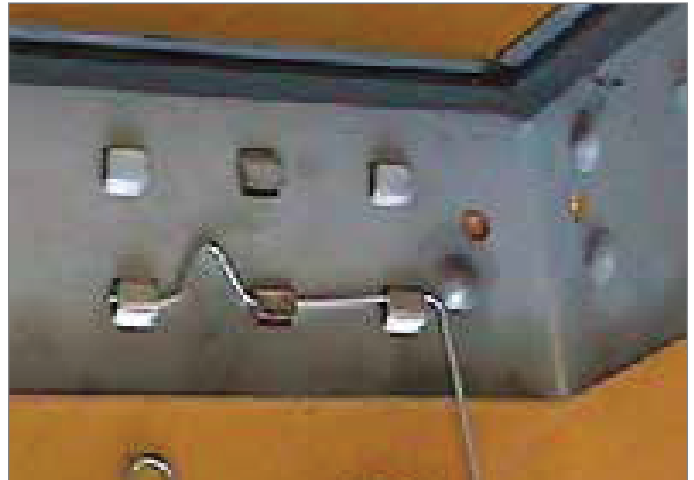
FIGURE 111 - CORRECTLY INSTALLED LATCH PIN (P/N 026-35788-604)
