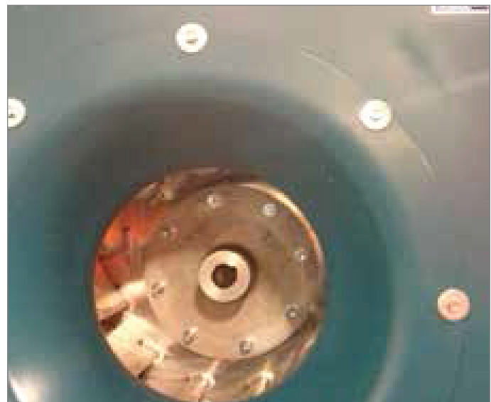
FIGURE 60 - PORT LOCATIONS FOR FAN MOUNTED AIR MONITORING SYSTEM
