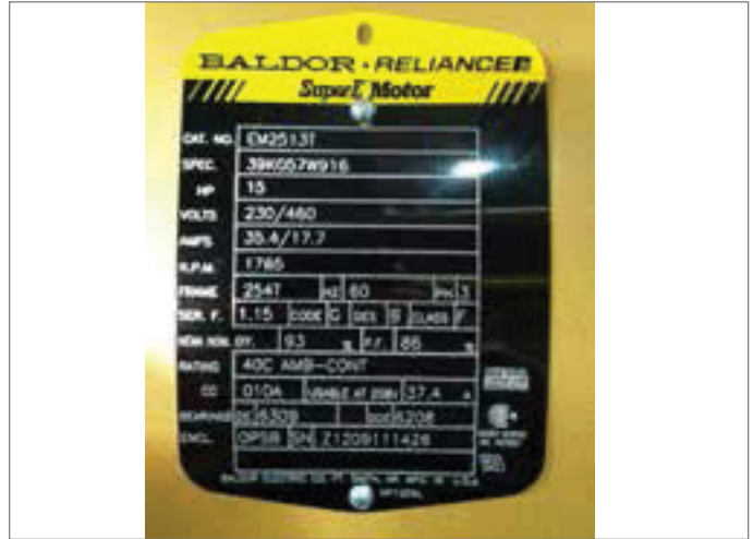
FIGURE 65 - ANOTHER TYPICAL MOTOR DATA / NAME PLATE
