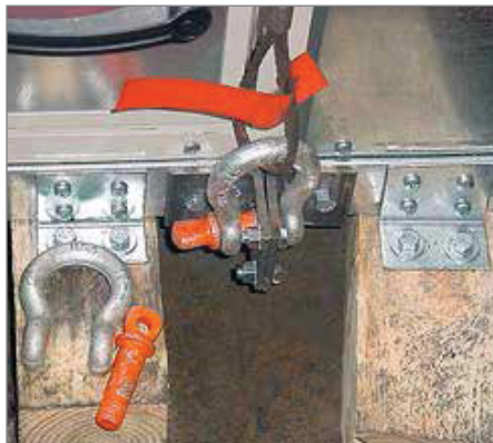
FIGURE 12 - PROPER LIFTING WITH SHACKLE AT LIFTING LUG
