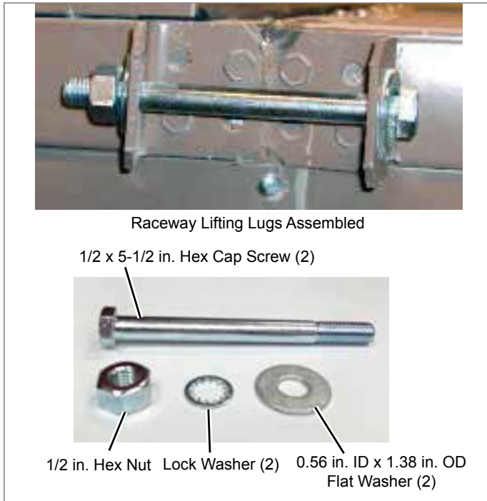
FIGURE 23 - TOP RACEWAY BRACKET ASSEMBLED (P/N 386-04747-000)
