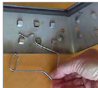
FIGURE 114 - CORRECTLY INSTALLED LATCH PIN (P/N 026-35788-604)
