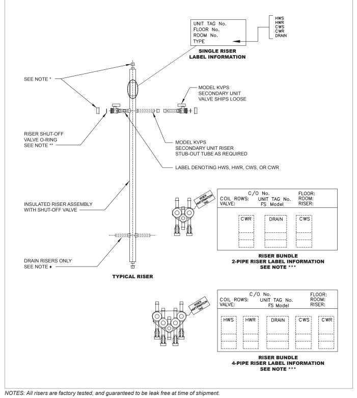
All risers and valves are shipped with protective caps. These caps should remain in place until installation of the unit.
