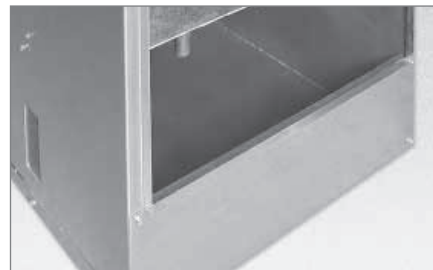
Positively sloped drain pan prevents standing water; lined with closed cell foam insulation for added moisture protection.
