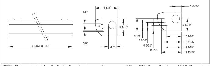
NOTES: All dimensions in inches. Cooling/heating water pipe connections are copper 1/2" and 3/8" with a wall thickness of 0.04". The maximum operating pressure of chilled/hot water pipework is 150 psi.
