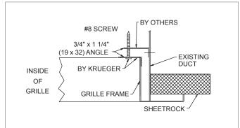
NOTES: Concealed mounting is not available with an OBD or with the 800/5800 series. Maximum unit size is 36"x20".
