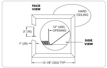
▼ ASDP/5ASDP/ASDT/5ASDT, FRAME 27, SPLINE, ADAPTER FRAME 24"x24" PANEL
