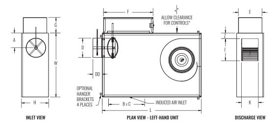
\* Check NEC for unit clearance requirements.
