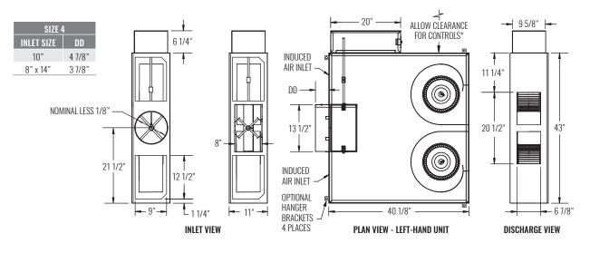
\* Check NEC for unit clearance requirements.
