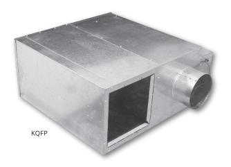
The Model KQFP features intermittent parallel fan operation and is designed to maintain optimum occupant comfort levels by supplying warm induced plenum air, cold primary air (VAV), or a mixture of both to condition the space. The fan cycles on to satisfy zone heating requirements. Optional electric or hot water heating coils provide terminal heat after the fan has cycled on.
