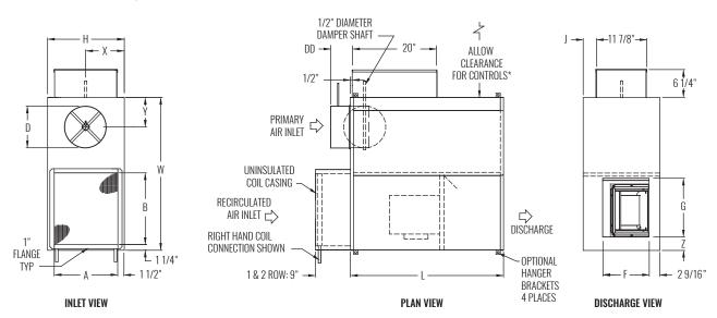
\* Check NEC for unit clearance requirements.
