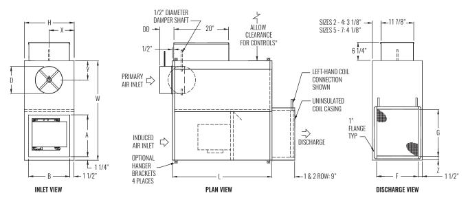
\* Check NEC for unit clearance requirements.
