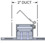
NOT COMPATIBLE WITH: 01 SPRING CLIPS 02 CONCEALED FASTENING DUCT WIDTH > 2" FRAME STYLES DS & RG
