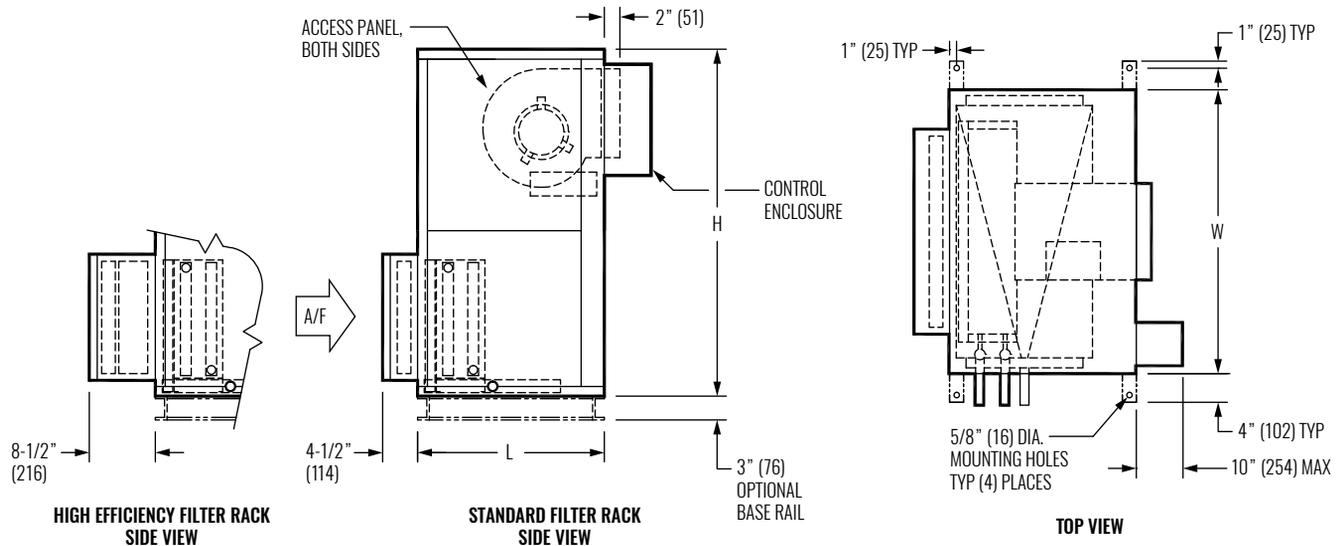
NOTES: Dimensions in parentheses are in millimeters (mm). See table below for dimensional references. Provide sufficient clearance to permit access to controls and comply with applicable codes and ordinances. Base rail is optional on the base unit. Base rails must be used with mixing box. Electric heaters are only available in fan arrangement 3.
