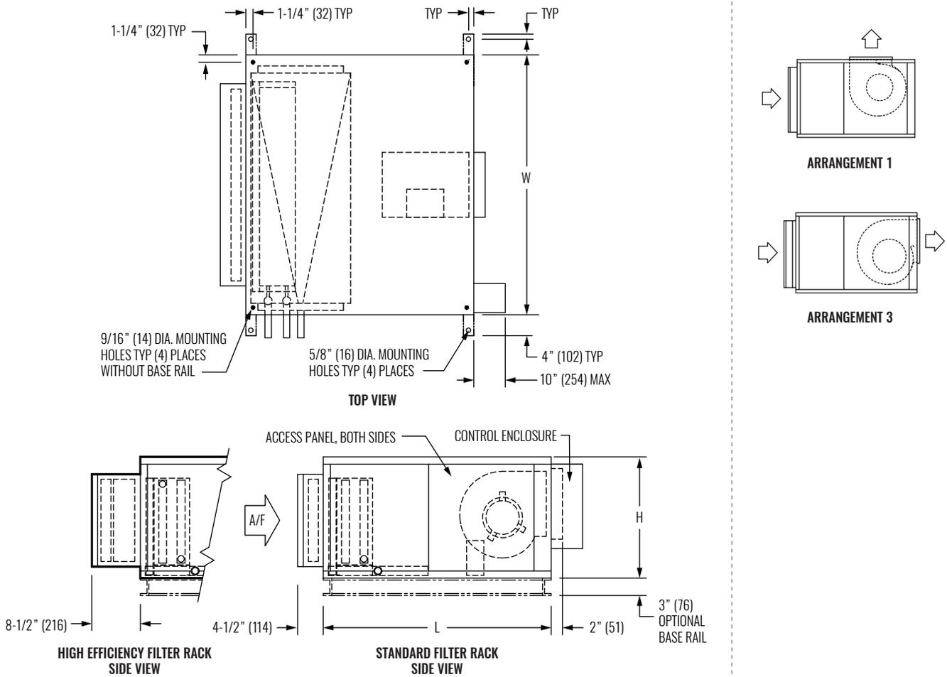
NOTES: Dimensions in parentheses are in millimeters (mm). See table below for dimensional references. Provide sufficient clearance to permit access to controls and comply with applicable codes and ordinances. Base rail is optional on the base unit. Base rails must be used with mixing box. Electric heaters are only available in fan arrangement 3.
