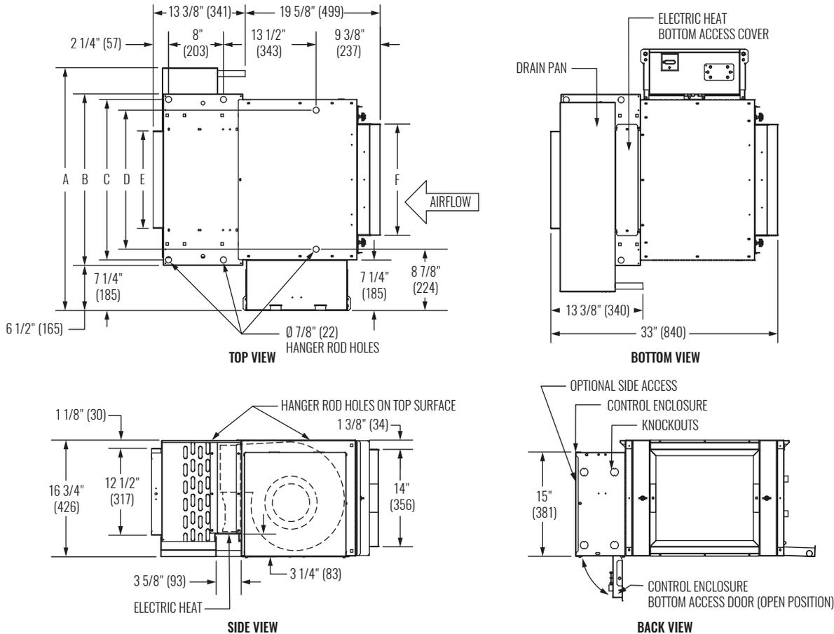
NOTES: Dimensions in parentheses are in millimeters (mm). See table below for dimensional references. The mixing box is field reversible from bottom to top and rear return. It is recommended to provide 3' access on pipe connection side. Provide access clearance for electrical enclosure per local and national electrical code requirements. Mixing box side panels are removable for access to the linkage / actuator.
