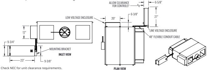
\* Check NEC for unit clearance requirements.
