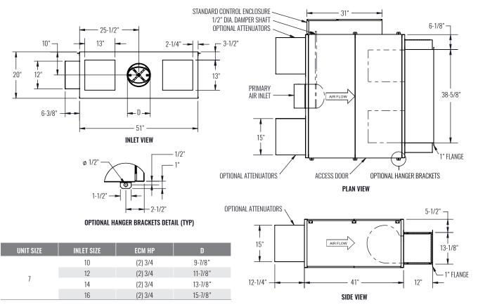
NOTES: Left-hand mounted controls shown above; right hand units (optional) are inverted, resulting in elevation change of discharge duct.
