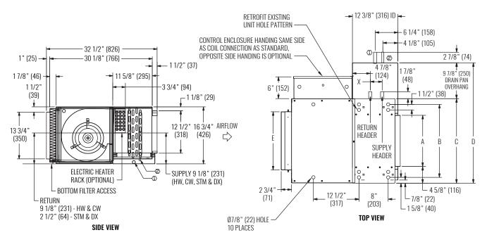
NOTES: Dimensions in parentheses are in millimeters (mm). See table below for dimensional references. The mixing box is field reversible from bottom to top and rear return. It is recommended to provide 3' access on pipe connection side. Provide access clearance for electrical enclosure per local and national electrical code requirements. Mixing box side panels are removable for access to the linkage / actuator.
