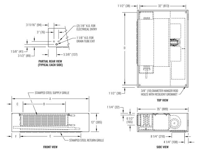
NOTE: Front stamped supply grille and bottom stamped return grille is shown. Other configurations are available. Left hand coil connection shown, right hand is available. Provide access clearance for electrical enclosure per local and national electrical code requirements. Dimensions in parentheses are in millimeters (mm). See table below for dimensional references.
