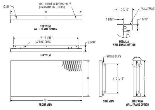
NOTES: Width (W) is 8" - 48" in 1" increments. Height (H) is 4" - 24" in 1" increments.
