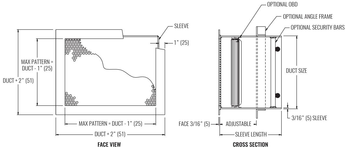
NOTES: Dimensions in parentheses are millimeters (mm). Recommended opening = duct size + 1/2". Optional angle frame or loose angles to be field welded for mounting.
