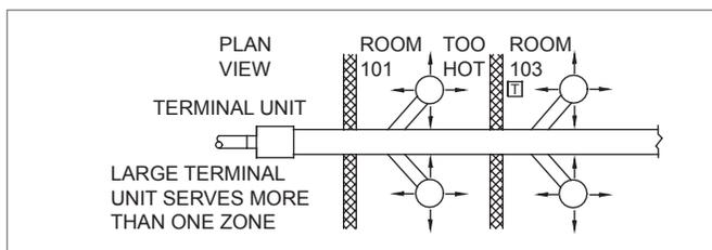
**NOTES:** When one large terminal unit serves a space that should be served by two or more smaller unit, comfort problems can result. There may be noticeable temperature differences between rooms, since the thermostat is located in just one room. Also, for a given air velocity, the larger the fan powered terminal, the more power it generates.
