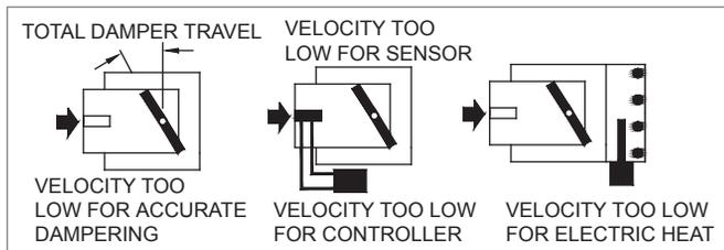
**NOTES:** The direct result of oversizing is low air velocity. With the velocity too low, the damper must operate in a pinched-down condition most of the time, making control difficult. The inlet velocity can also be too low for effective operation of the sensor and controller. Too low a velocity through an electric heater will cause the safety airflow switch to shut down the heater.
