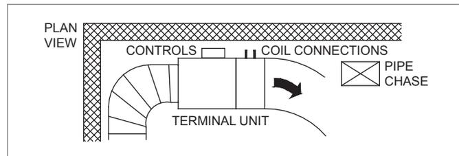
**NOTES:** Carefully planning the locations of the terminals avoids problems with installation, performance, and maintenance. The control side of the terminal is against the wall, making connections difficult and service impossible. The cramped location also creates the need for close-coupled duct elbows, which reduce performance.
