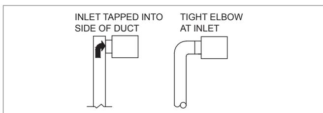
**NOTES:** The arrangement of duct at the terminal inlet affects both pressure drop and control accuracy. The conditions shown (left) will create turbulence at the inlet. This makes it difficult for the sensor to measure airflow. Although Krueger velocity sensors correct for a considerable amount of turbulence, the best practice is to use straight duct at the inlet.
