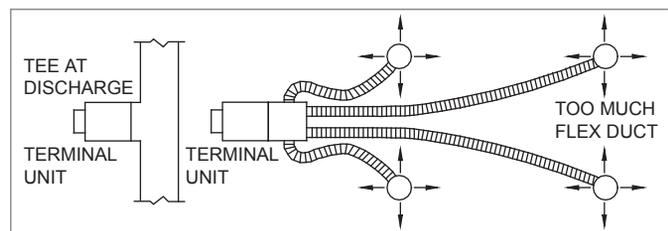
**NOTES:** The duct connections at the discharge end of the terminal have a major affect on pressure drop. A tee close to the discharge should be avoided, along with transition pieces and elbows. Another common error is running too much flex duct. It would have been better to continue the rectangular duct to the last diffuser, then install short flex branches.
