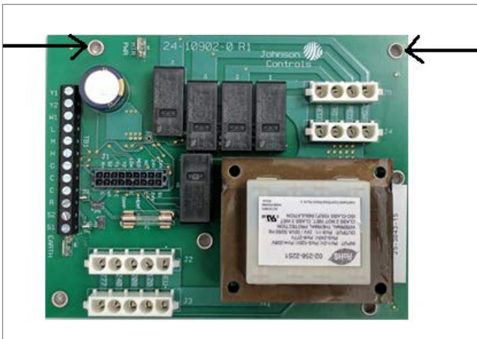
Figure 12 – FRBii mounting holes to align
