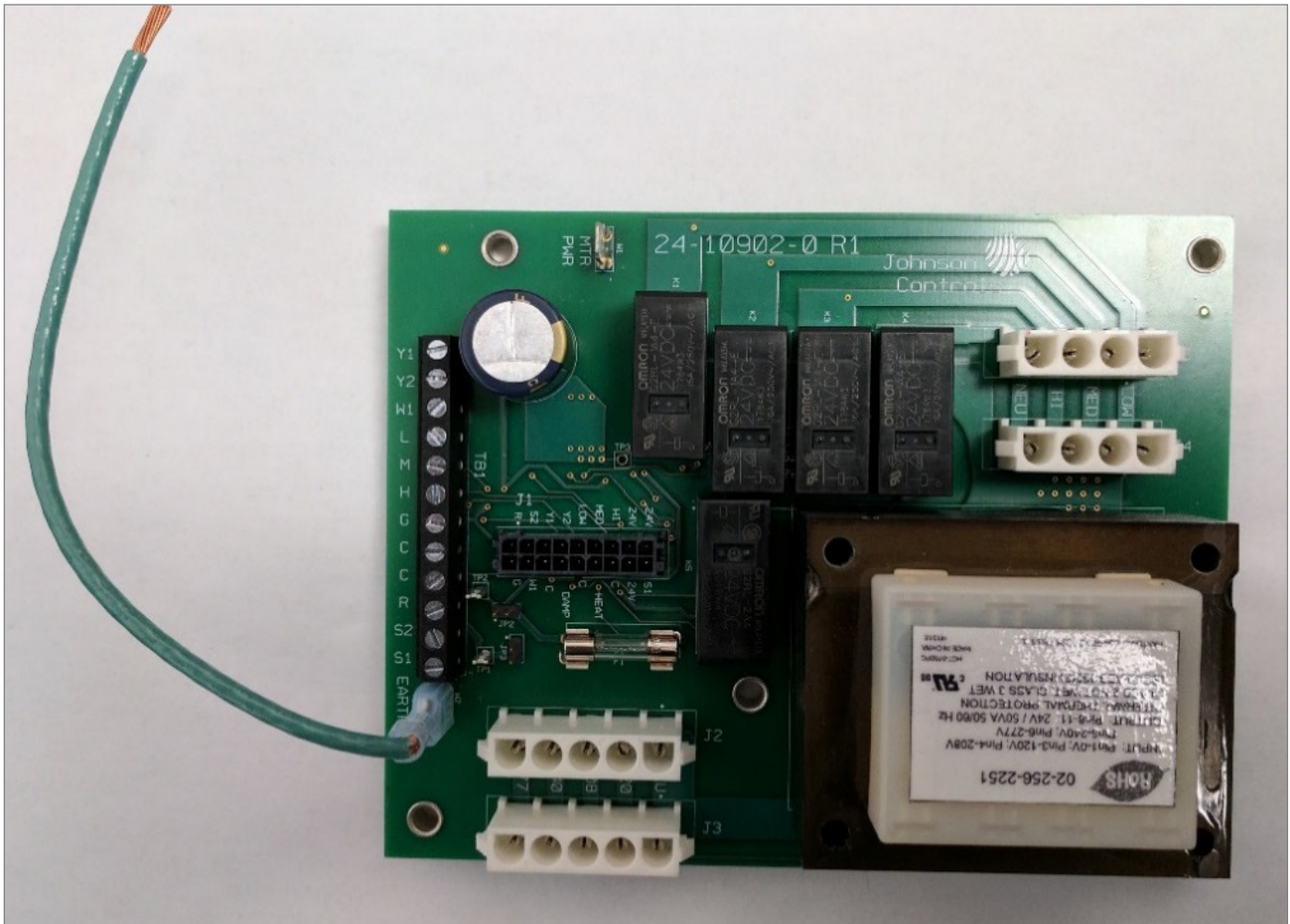
Figure 22 - Install WH1 on EARTH of FRBii
