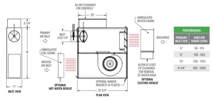
NOTES: Left-hand unit with electronic control enclosure shown; right-hand is available. Discharge requires flanged duct; connection by others. See table below for dimensional references.
