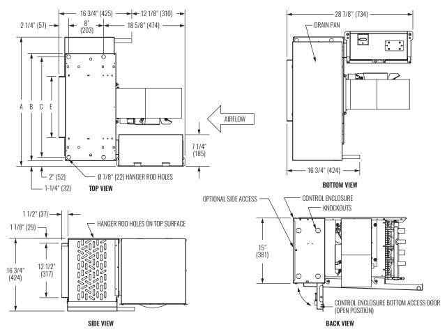
NOTE: Left hand coil shown, right hand is available. Provide access clearance for electrical enclosure per local and national electrical code requirements. Dimensions in parentheses are in millimeters (mm). See table below for dimensional references.
