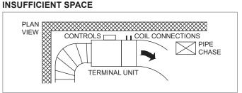
NOTES: Carefully planning the locations of the terminals avoids problems with installation, performance, and maintenance. The control side of the terminal is against the wall, making connections difficult and service impossible. The cramped location also creates the need for close-coupled duct elbows, which reduce performance.
