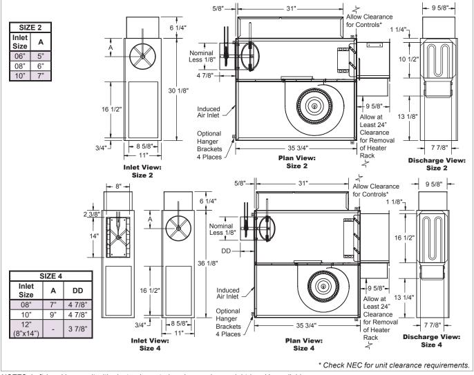
NOTES: Left-hand base unit with electronic control enclosure shown; right-hand is available. See page B2-124 for electric heat standard features.
