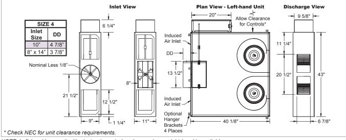
NOTE: Left-hand base unit with electronic control enclosure shown; right-hand is available.
