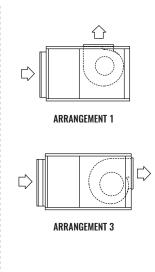
NOTES: Dimensions in parentheses are in millimeters (mm). See table below for dimensional references. Provide sufficient clearance to permit access to controls and comply with applicable codes and ordinances. Base rail is optional on the base unit. Base rails must be used with mixing box. Electric heaters are only available in fan arrangement 3.
