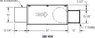
NOTES: Left-hand mounted controls shown above; right hand units (optional) are inverted, resulting in elevation change of discharge duct.
