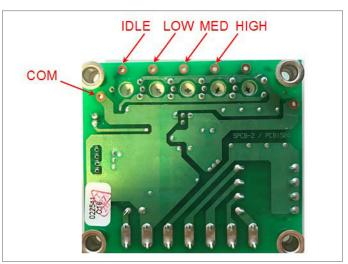
FIGURE 4 - Select PWM Test Points (back)
