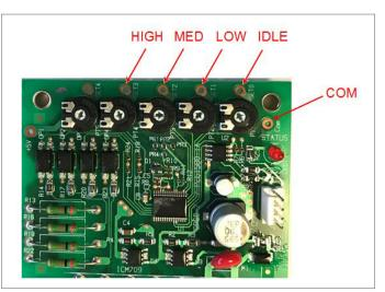
FIGURE 3 - Select PWM Test Points (front)
