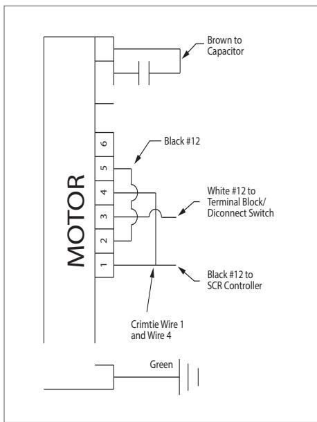
FIGURE 14 – PSC Motor Wiring Terminal Block –
