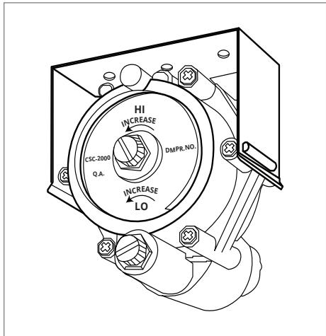
FIGURE 10 – Pneumatic Single Function Volume Controller (Normally Open) for Pneumatic Control Unit (Beige Color)
