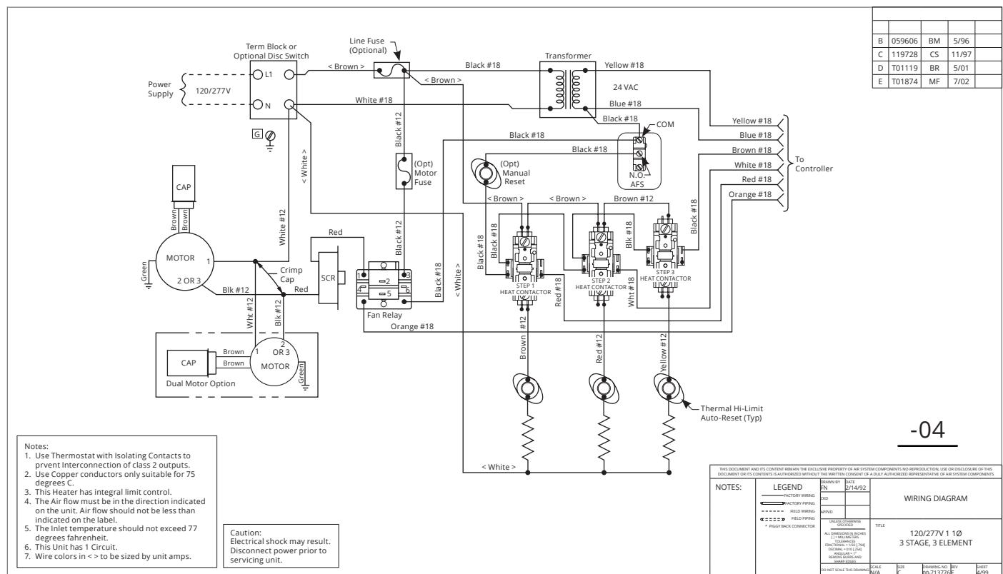
FIGURE 7 – Typical Power Connections for Fan Powered Units with 3-Stage Electric Heat
