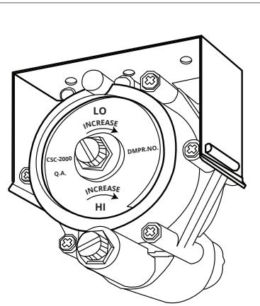
FIGURE 11 – Pneumatic Single Function Volume Controller (Normally Closed) for Pneumatic Control Unit (Grey Color)
