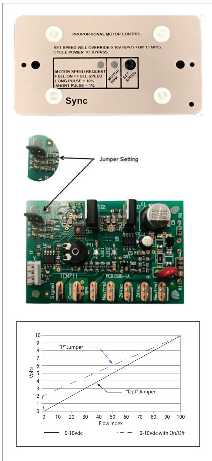
FIGURE 11 – Remote Speed, ECM Controller
