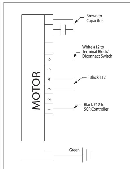
FIGURE 17 – PSC Motor Wiring Terminal Block –
