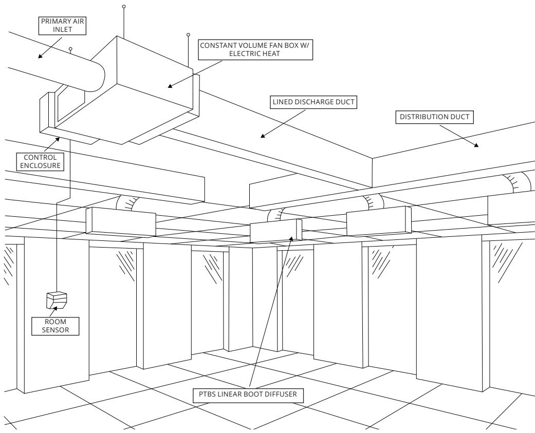
FIGURE 6 – Typical Perimeter Installation – Constant Volume Fan-Powered Box
