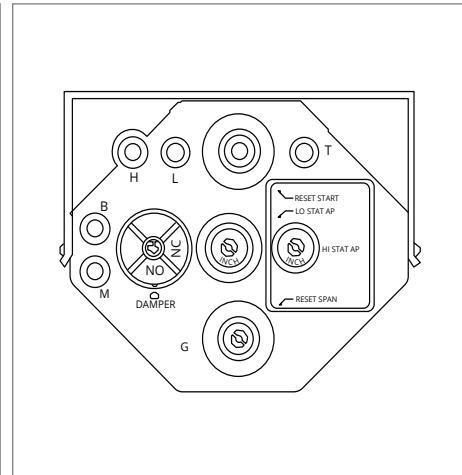
FIGURE 12 – Multi-Function Reset Volume Controller
