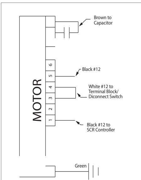
FIGURE 15 – PSC Motor Wiring Terminal Block –
