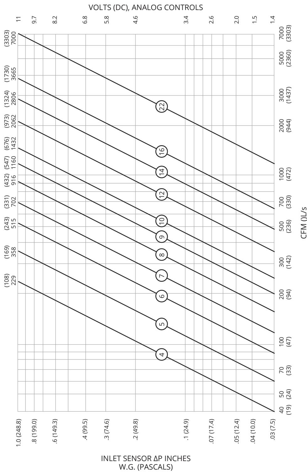
FIGURE 8 – Inlet Airflow Sensor CFM vs. Signal Chart
