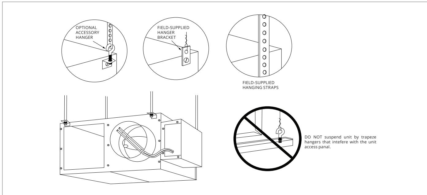
*FIGURE 5 – Typical Unit Suspension Methods (KQFP Shown)*
